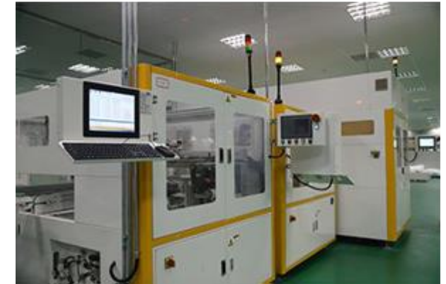
EL tester & Visual inspection instrument
